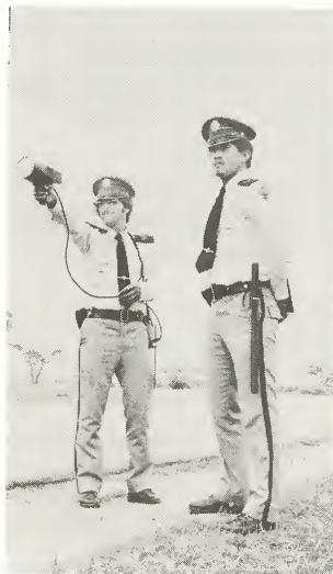
In one of the TV programs, traffic police are seen measuring the speed of an oncoming motor vehicle with a radar drum. The apparatus has a locking device which permits the driver to see at which speed he had been driving. Drivers found to exceed speed limits during surprise spot checks are fined.
